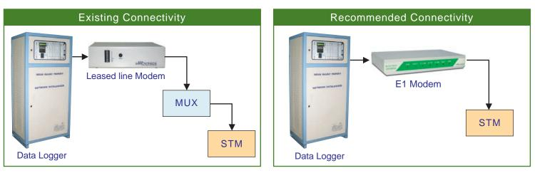
With E1 connectivity we can completely remove the need of primary multiplexer. This creates less number of connections and improves reliability of Datalogger network further. Failures of mux are comparatively high. So elimination mux will improve network connectivity.
